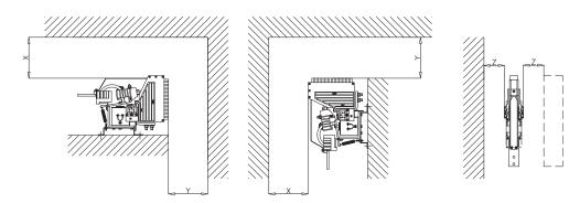
Minimum clearances from metal parts [mm] X = 80; Y = 210; Z = 40
